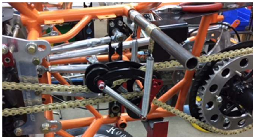
Figure 11 Spring hangers mounted and springs mounted to hangers
