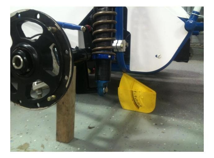
NOW I HAVE MOVED TO THE FRONT AND I WANT THIS MEASUREMENT  $\frac{1}{4}$  TO  $\frac{1}{2}$  INCH HIGHER THAN THE REAR.
