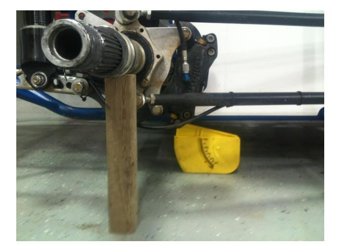
ALWAYS MEASURE IN THE SAME PLACE, I HAVE STARTED USING THIS GROUND CLEARANCE MEASUREMENT WHICH IS RIGHT UNDER THE FIRST AND LAST VERTICAL UPRIGHTS IN THE CHASSIS. THIS IS WHAT I CALL GUAGE HEIGHT OR GUAGE BLOCK HEIGHT. I HAVE STARTED USING THIS MEASUREMENT SO TUBE HEIGHTS DON'T COME INTO PLAY.
