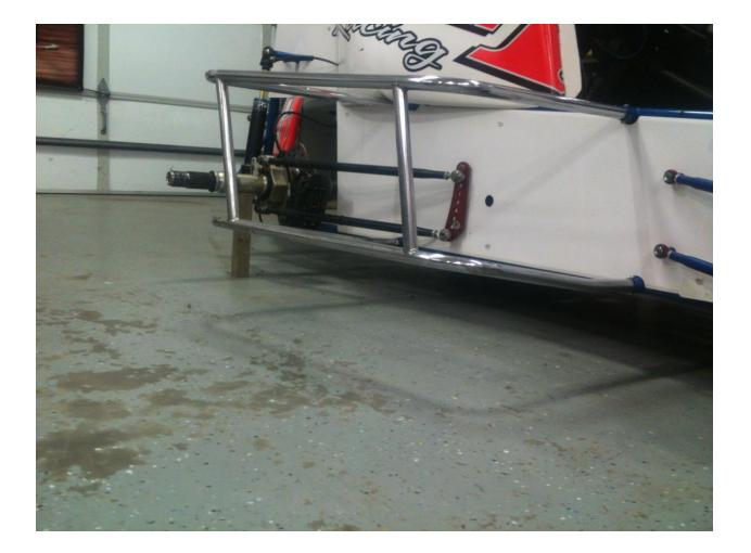
THIS SHOWS OUR 4 LINK SET UP WITH THE #41 REAR ADJUSTABLE RADIUS ROD PLATE – ANOTHER GREAT ADJUSTMENT FOR CHANGING TRACKS.
